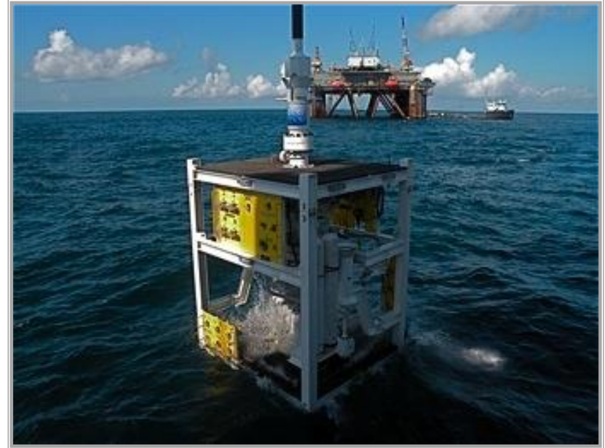
Deploying Blue Ocean Technologies subsea well intervention equipment from the HOS Iron Horse
