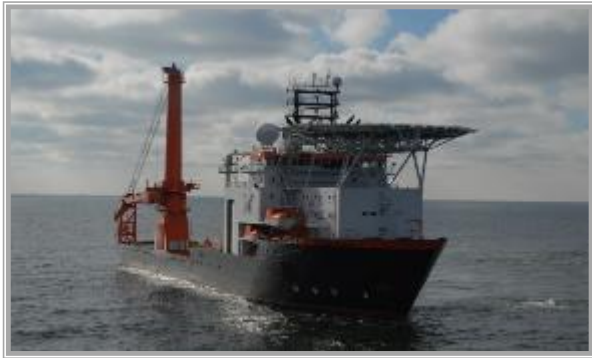
HOS Iron Horse , our second of two 430-ft foreign-built DP3 Merwede T-22 class MPSVs
