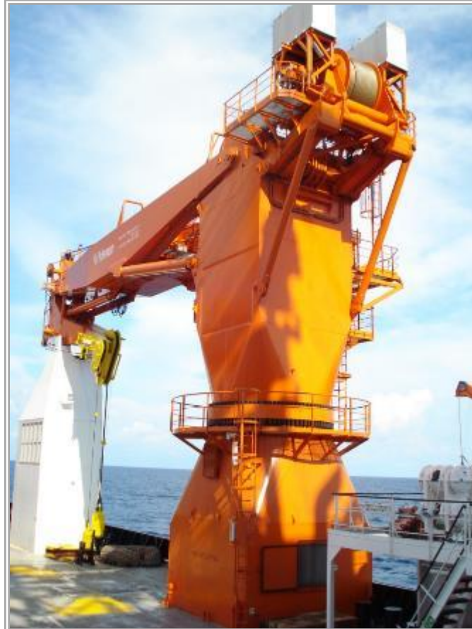
120-ton knuckle-boom crane on the HOS Iron Horse
