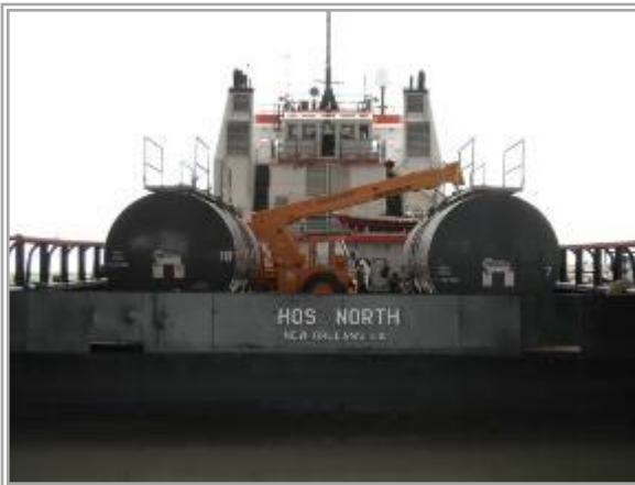
The HOS North configured as an oil skimming vessel with portable marine tanks
