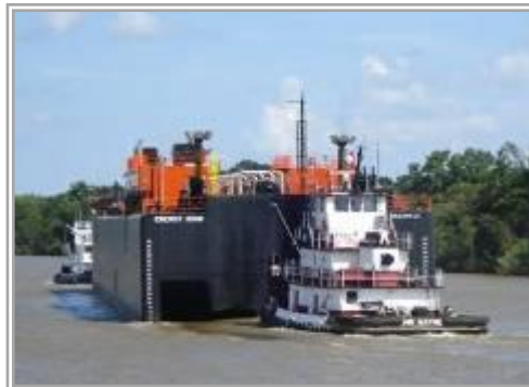
Energy 6506 , our first 60,000-bbl double-hulled tank barge newbuild
