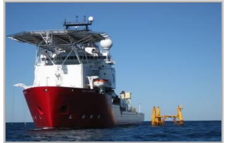
DP3 T-22 class MPSV, HOS Achiever , on her first shelf platform remediation job in the GoM after Hurricanes Gustav and Ike in 2008
