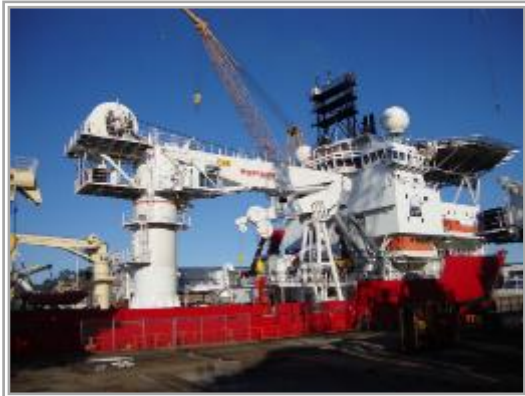
100-ton knuckle-boom crane on the HOS Achiever
