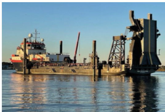
HOS Resolution configured into amphibious landing vessel
