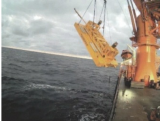
HOS Warland Setting Subsea Equipment
